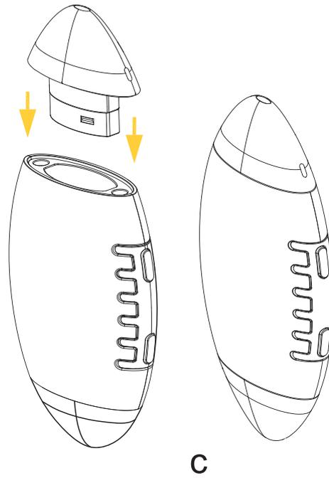
3. The pod and the nozzle is designed for the card slot, To remove the pod easily , we should shake it on the left and right promote. Shake it first on one promote and hear the sound, and then you shake the other promote and also hear the sound, so that it will be easy to remove the pod.
